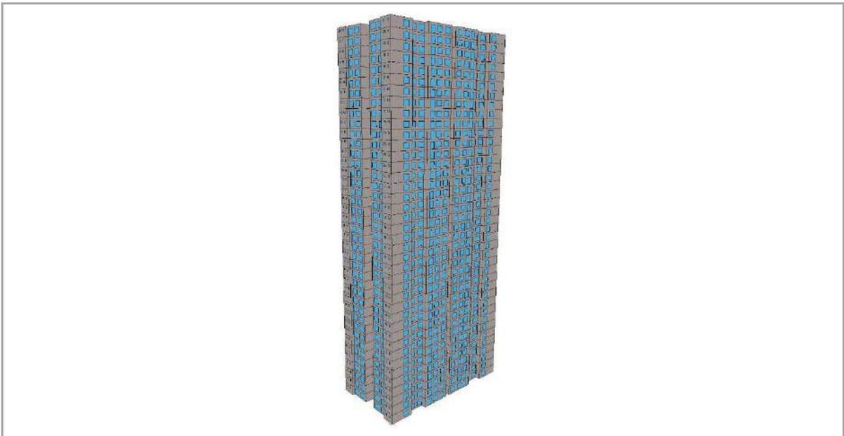
The project has been modelled with the e-QUEST energy analysis software that uses the DOE 2.2 Building energy simulation engine. The e-QUEST energy modelling software allows for a graphical display of all the 3-dimensional geometry entered in the application to describe the building. As per the view shown, the Building has been modelled in detail to improve the accuracy of analysis work.
